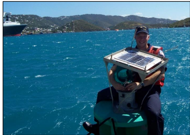
Figure 5: Ubiquitous energy harvesting system present in waterways across the globe. Here, a buoy fitted with a 155mm lantern and 10W solar panel is being repaired in St. Thomas, USVI after a vessel collided with it [17].
